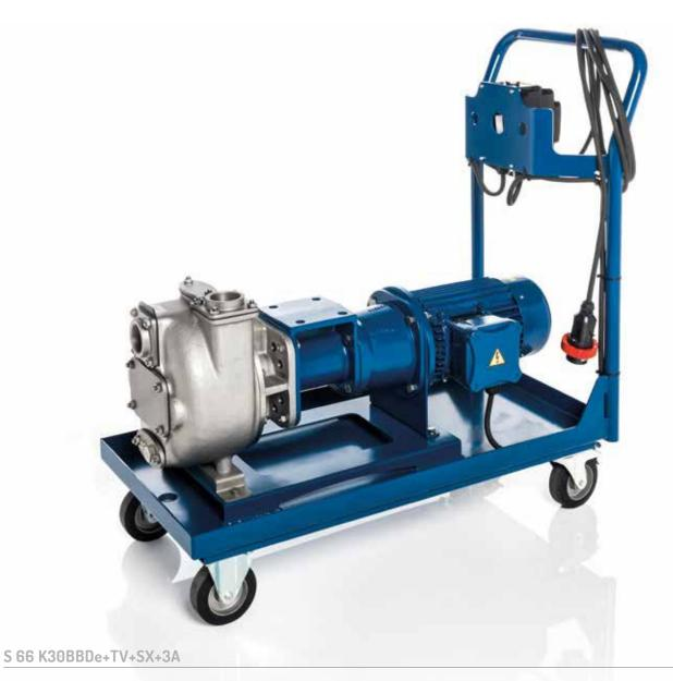
Stainless steel pump with 2" threaded ports, Bi-Block build with electric cable, on/off switch, with 4-wheeled trolley suitable for flat ground.
